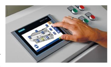
Recipe management, airflow, table angle, in-feed and vibration speed can all be adjusted with the user friendly touch panel. All settings can be saved allowing for exceptional and repeatable sorting results.
